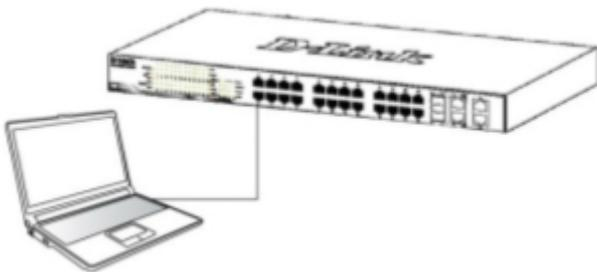
2. Configure the PC's IP address to be in the network segment as the switch. The switch's default IP address is 10.90.90.90 with a subnet mask of 255.0.0.0 and a default gateway of 0.0.0.0. For example, to connect to the switch using the default settings, your PC should have an IP address in the range: 10.0-255.0-255.1-254 and a subnet mask of 255.0.0.0.
