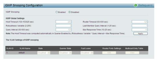
Figure 5.50 - Configuration > IGMP Snooping > IGMP Snooping
