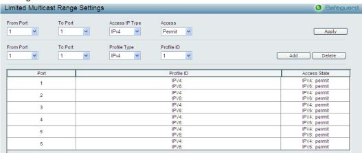
$Figure \ 5.58 \hbox{-}\ Configuration > IGMP\ Snooping > Limited\ Multicast\ Range\ Settings$
