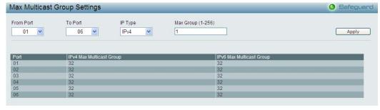
$Figure \ 5.59-\ Configuration > IGMP\ Snooping > Max\ Multicast\ Group\ Settings$
