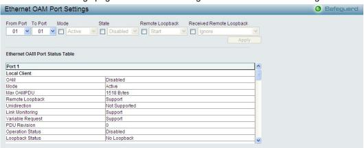
Figure 5.70 - Configuration > Ethernet OAM > Ethernet OAM Port Settings
