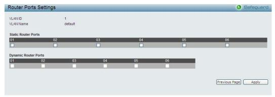
Figure 5.51 - Configuration > IGMP Snooping > IGMP Snooping-Router Port Settings
