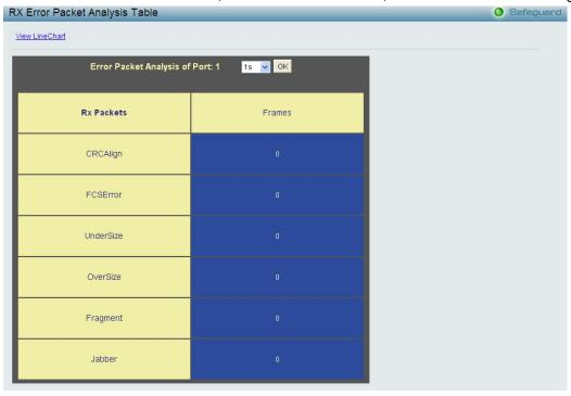
$Figure \ 5.119 \ \textbf{-} \ Monitoring > Errors > Received \ (RX) \ (table)$
