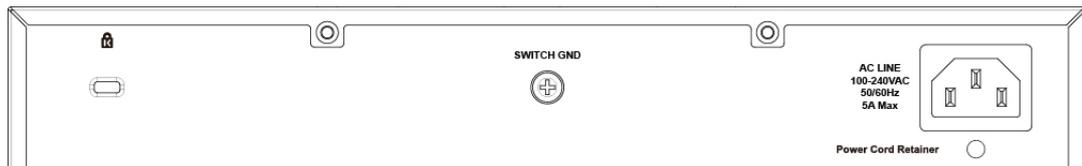
Figure 2-4 DGS-1100-10MPP Rear Panel
