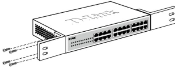
**Figure 3-2 Attach the mounting brackets to the switch**
