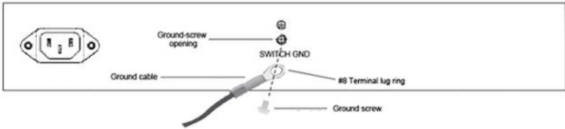
Figure 3-5 Ground cable, screw and #8 terminal lug rings
