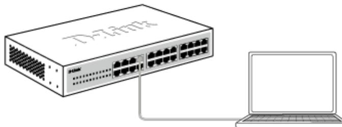
Figure 4-1 Connecting to a DGS-1100 MP/MPP Series switch
