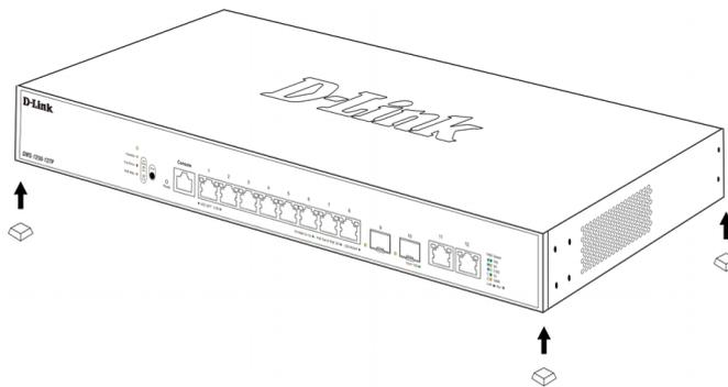
**Figure 1 — Attaching rubber feet to the Switch**
