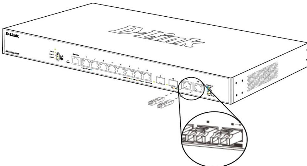
Figure 4 — Inserting transceivers into the transceiver ports
