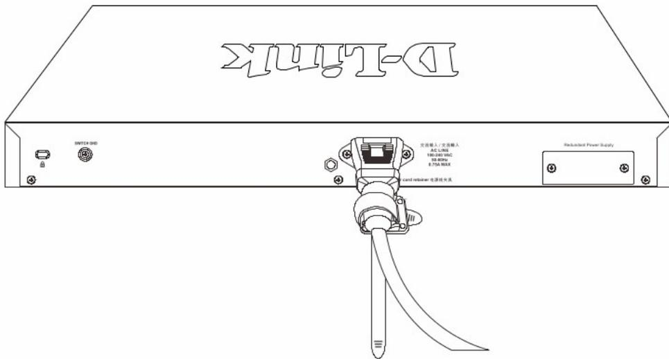
Figure 9 — Secure the power cord
