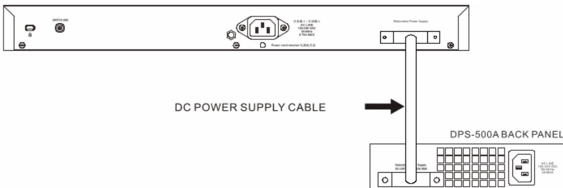
Figure 10 — Connecting the Switch to the DPS-500A
