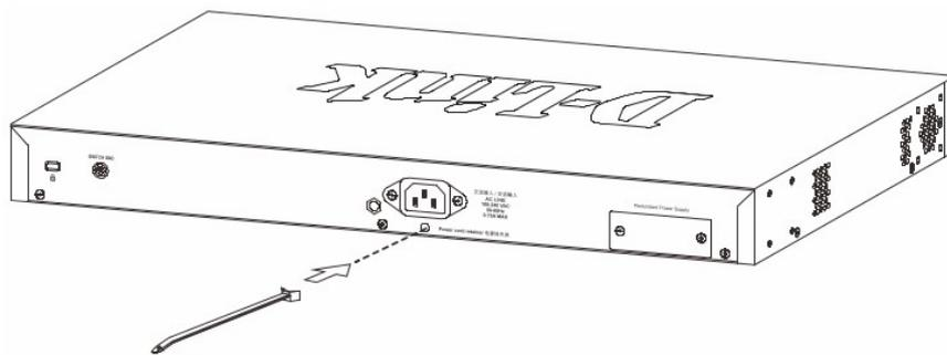
**Figure 5 — Insert Tie Wrap into the Switch**
