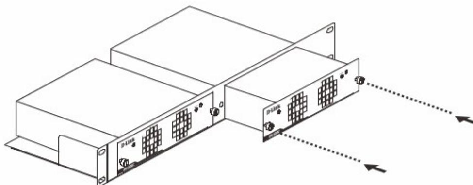
**Figure 11 — Install the DPS-500A in the DPS-800**
