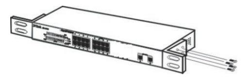
Figure 2. Combine the Switch with the provided screws
