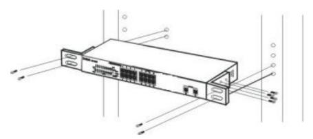
Figure 3. Mount the Switch in the rack
