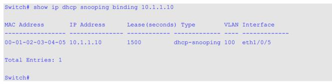
This example shows how to display DHCP snooping binding entries by IP 10.1.1.10 and MAC 00-01-02-00-00-05.
