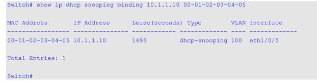
This example shows how to display DHCP snooping binding entries by IP 10.1.1.10 and MAC 00-01-02-03-04-05 on VLAN 100.
