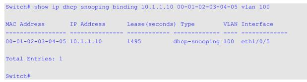
This example shows how to display DHCP snooping binding entries on port 5.
