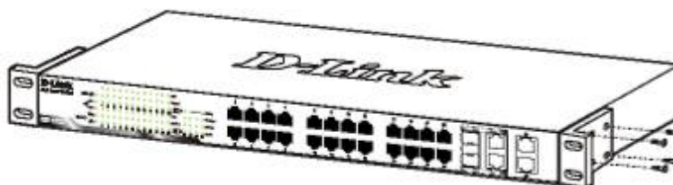
Figure 2.2 – Attach the mounting brackets to the Switch
