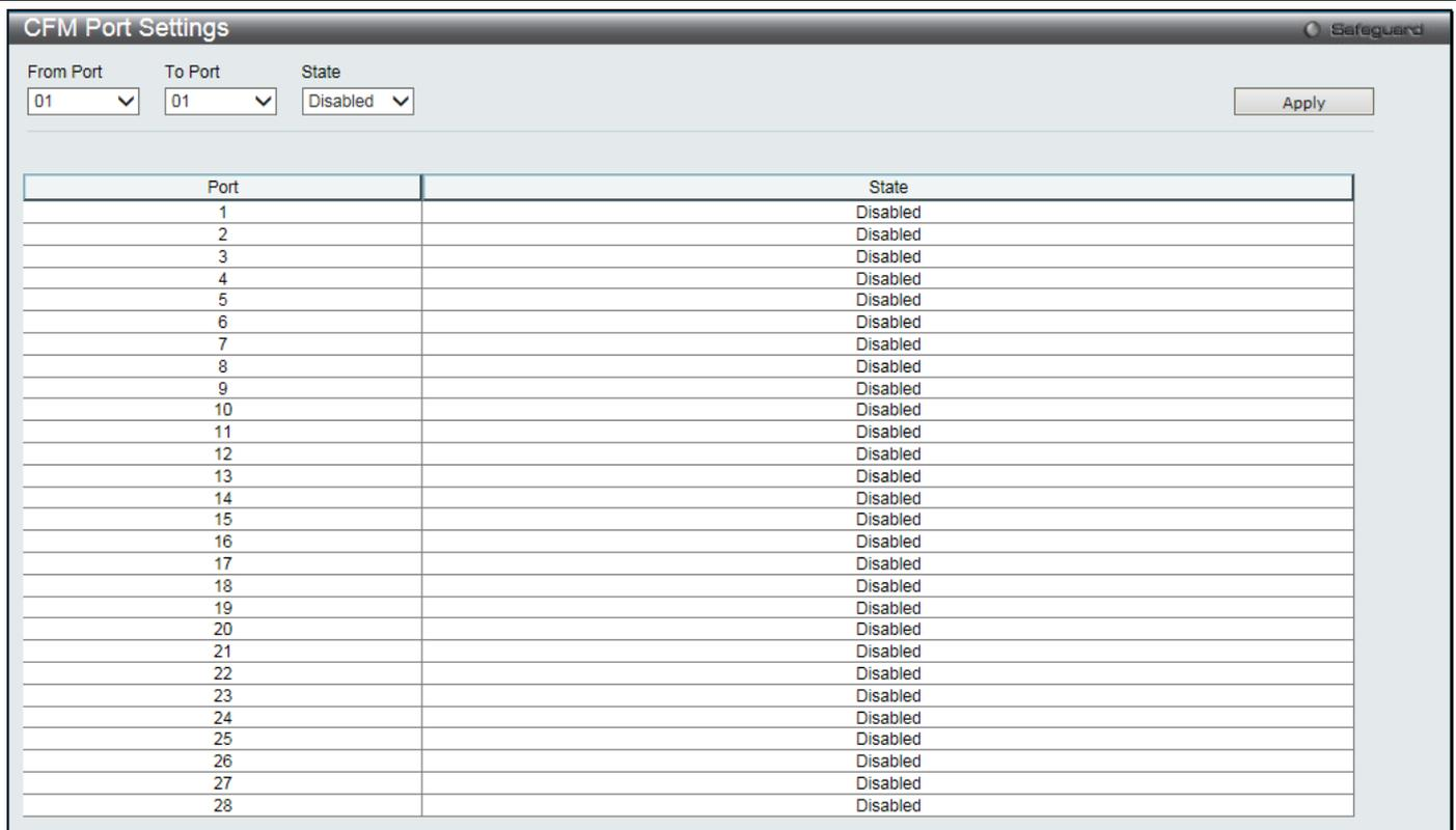
The screenshot shows the 'CFM Port Settings' window. At the top, there are three dropdown menus: 'From Port' (set to 01), 'To Port' (set to 01), and 'State' (set to Disabled). An 'Apply' button is located to the right of these menus. Below the menus is a table with two columns: 'Port' and 'State'. The table lists ports from 1 to 28, all of which are currently set to 'Disabled'.
