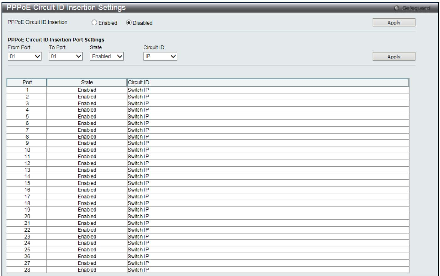
Figure 9-16 PPPoE Circuit ID Insertion Settings window
