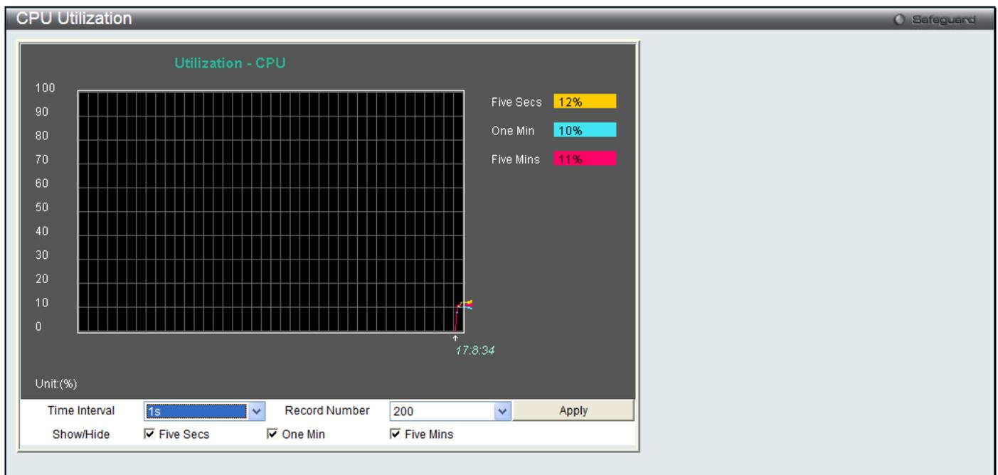
Figure 11-1 CPU Utilization window
