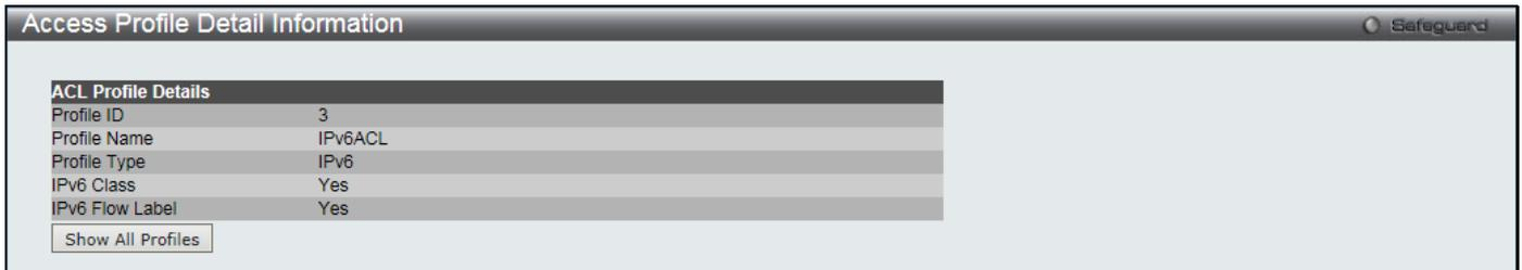
**Figure 7-14 Access Profile Detail Information window (IPv6 ACL)**
