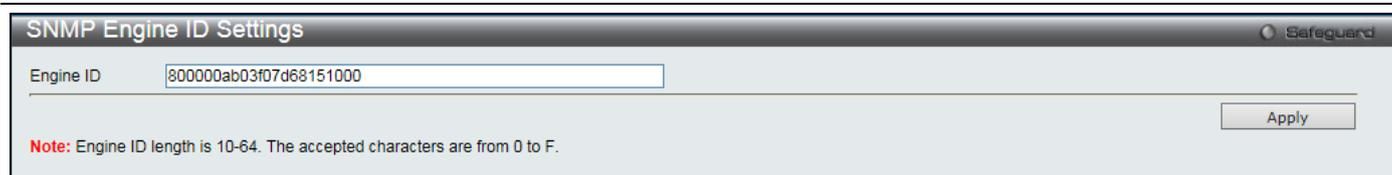
The screenshot shows the 'SNMP Engine ID Settings' window. At the top, there is a text input field for 'Engine ID' containing the value '800000ab03f07d68151000'. To the right of the input field is an 'Apply' button. Below the input field, a red note states: 'Note: Engine ID length is 10-64. The accepted characters are from 0 to F.'
