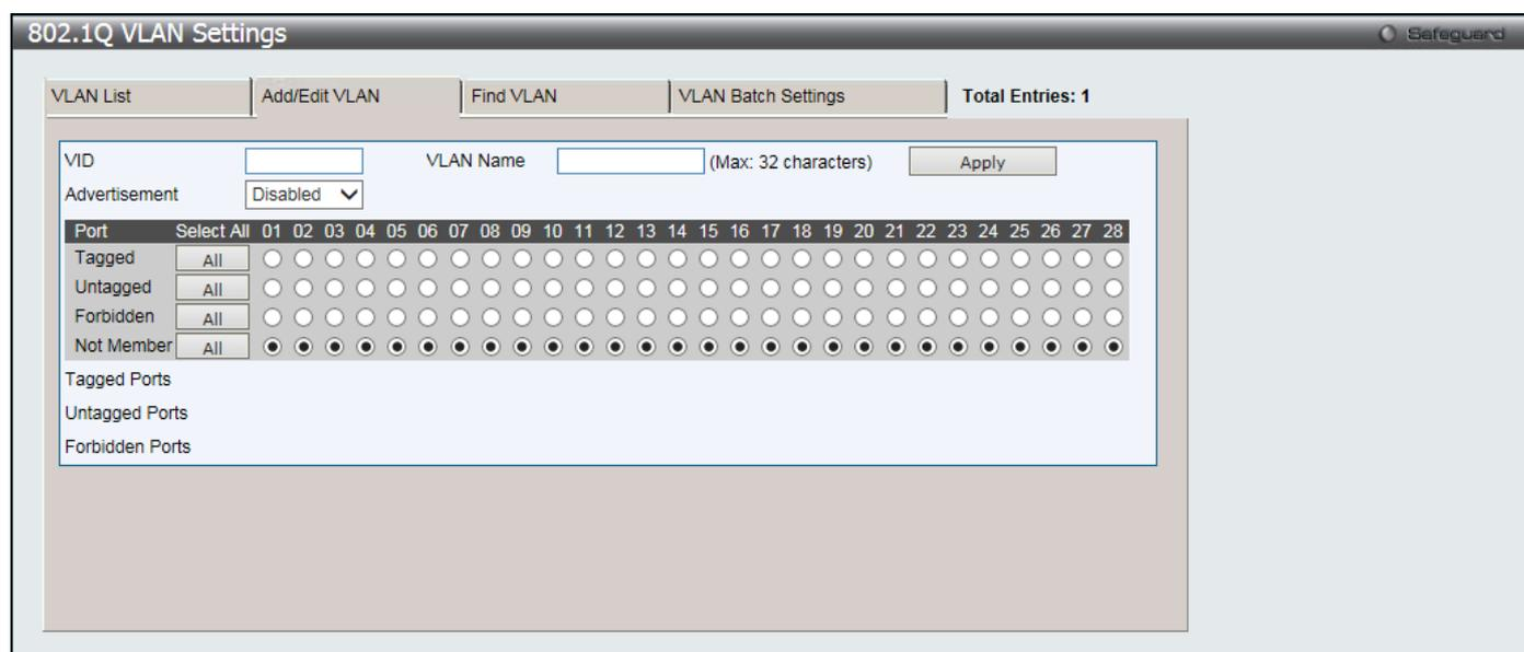
Figure 4-5 802.1Q VLAN Settings – Add/Edit VLAN Tab window
