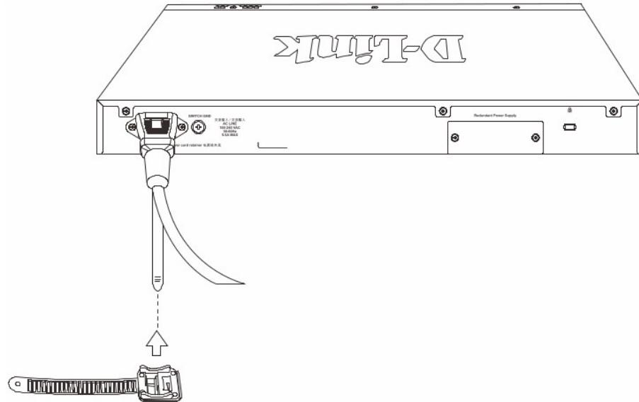
**Figure 10 — Slide the retainer through the tie wrap**
