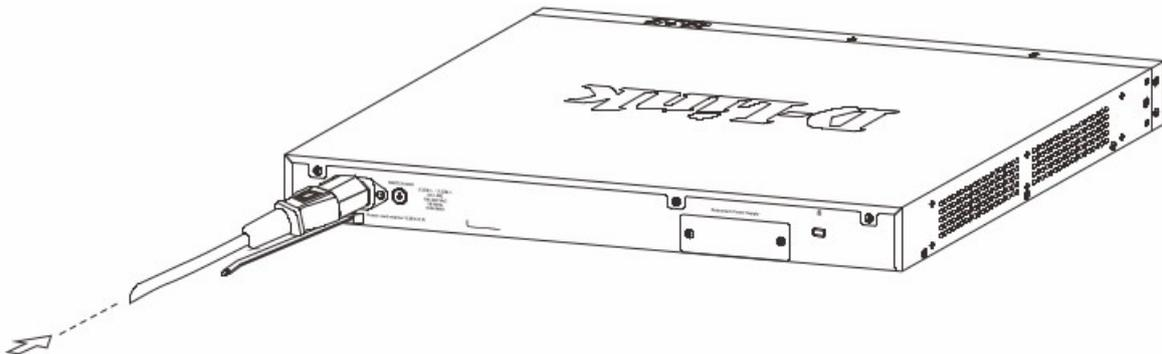
**Figure 9 — Connect the power cord to the switch**
