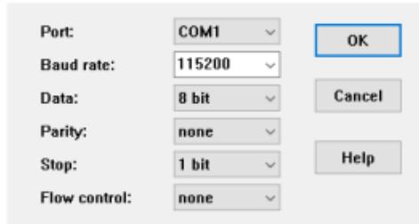
Figure 14 — COM port configuration
