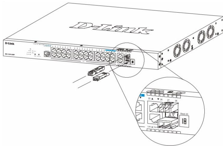
**Figure 7 — Inserting transceivers into the transceiver ports**
