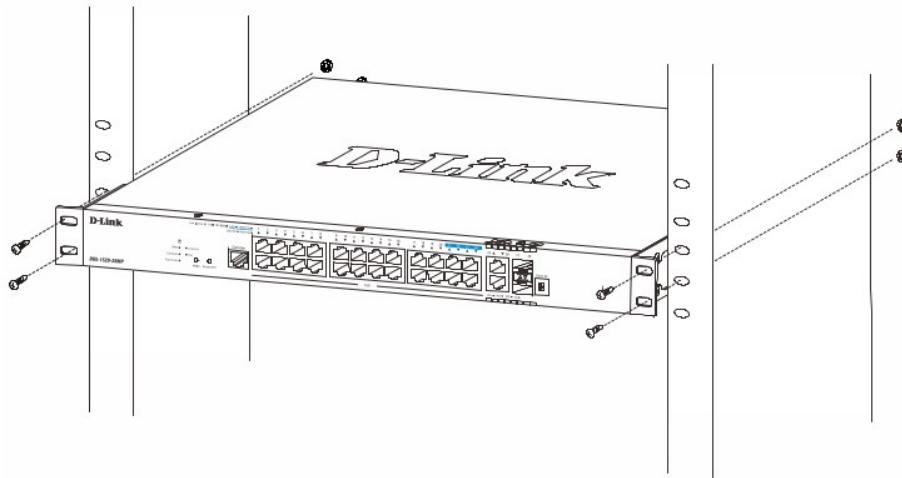
**Figure 6 — Installing the switch in a rack**
