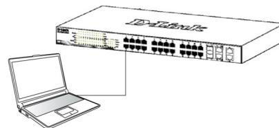
2. Configure the PC's IP address to be in the network segment as the switch. The switch's default IP address is **10.90.90.90**, with subnet mask **255.0.0.0**.
