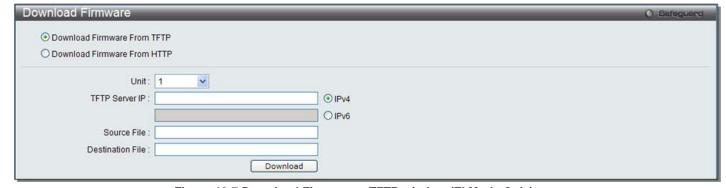
Figure 12-7 Download Firmware – TFTP window (El Mode Only)
