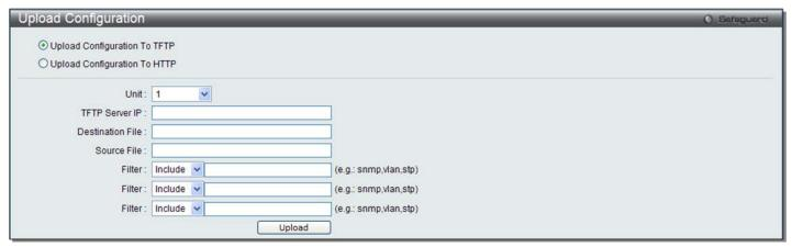
Figure 12-14 Upload Configuration – TFTP window (SI Mode Only)
