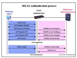
Figure 8-6 The 802.1X Authentication Process
