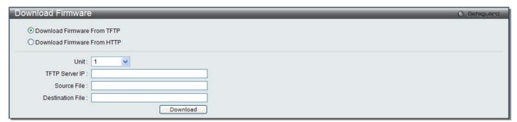
Figure 12-6 Download Firmware – TFTP window (SI Mode Only)
