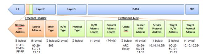
A common DoS attack today can be done by associating a nonexistent or any specified MAC address to the IP address of the network's default gateway. The malicious attacker only needs to broadcast one Gratuitous ARP to the network claiming it is the gateway so that the whole network operation will be turned down as all packets to the Internet will be directed to the wrong node.
