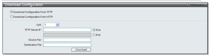
Figure 12-12 Download Configuration - TFTP window (El Mode Only)
