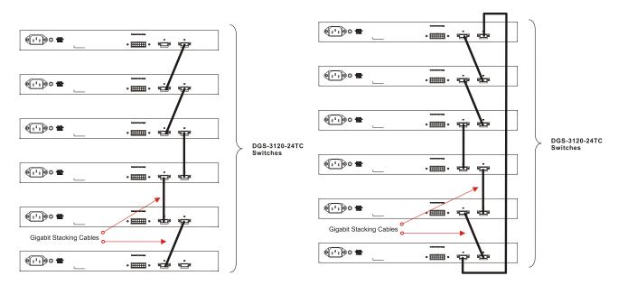
Figure 2-32 Switches stacked in a Duplex Chain
