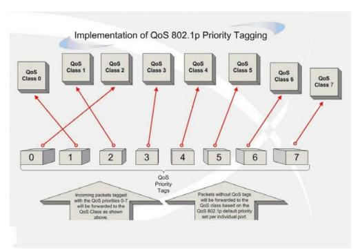
Figure 6-1 Mapping QoS on the Switch
