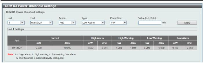
Figure 10-282 DDM RX Power Threshold Settings Window
