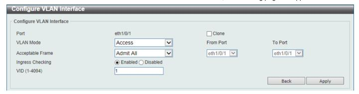
Figure 5-21 VLAN Interface (Access) Window
