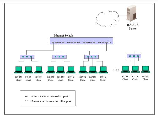
Figure 9-11 Example of Typical Host-based Configuration
