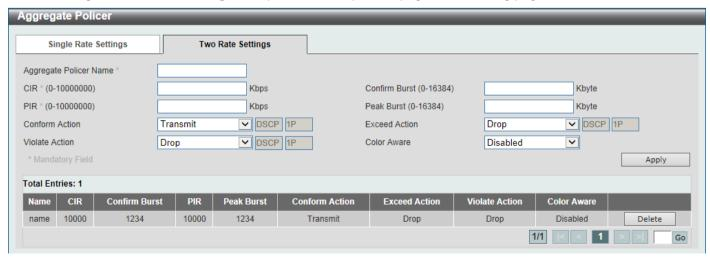
Figure 7-15 Aggregate Policer (Two Rate Settings) Window
