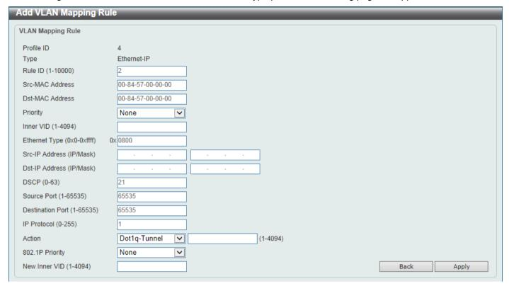
Figure 5-45 VLAN Mapping Profile (Ethernet-IP, Add Rule) Window
