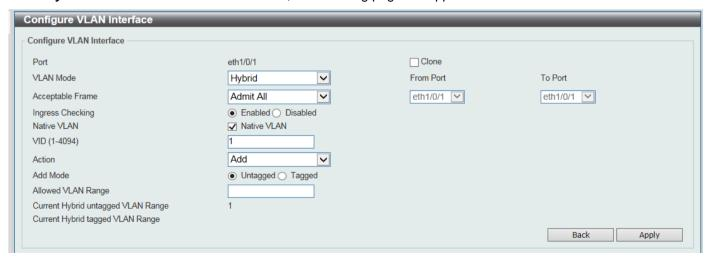
Figure 5-22 VLAN Interface (Hybrid) Window
