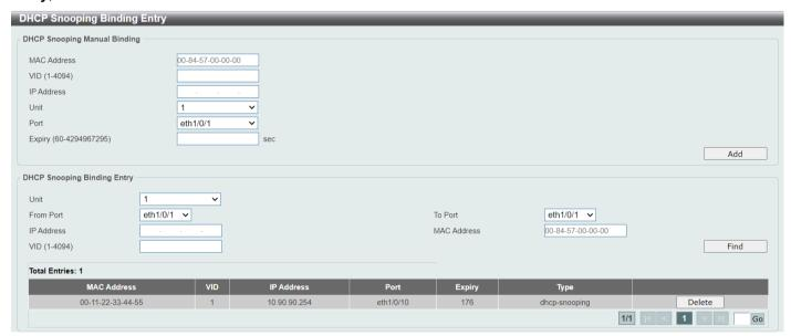
Figure 9-43 DHCP Snooping Binding Entry Window
