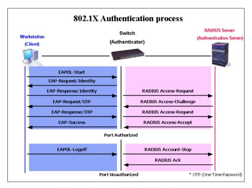
Figure 9-9 The 802.1X Authentication Process
