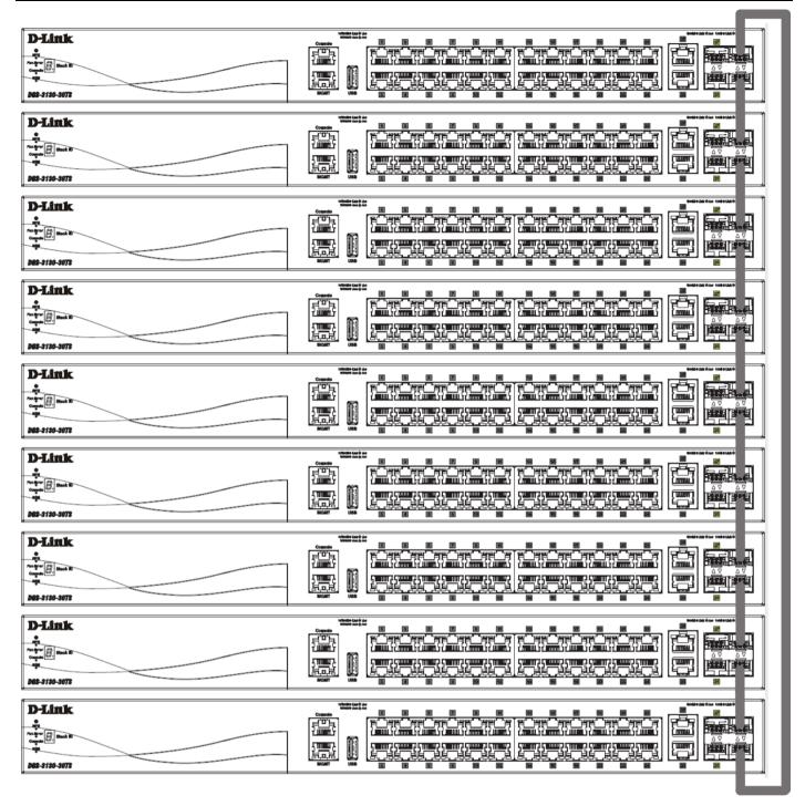
Figure 4-69 Duplex Ring stacking topology (SFP+)
