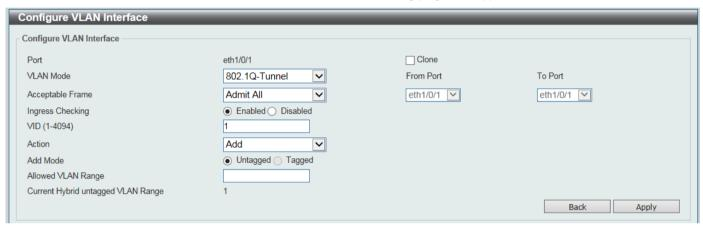
Figure 5-24 VLAN Interface (802.1Q-Tunnel) Window
