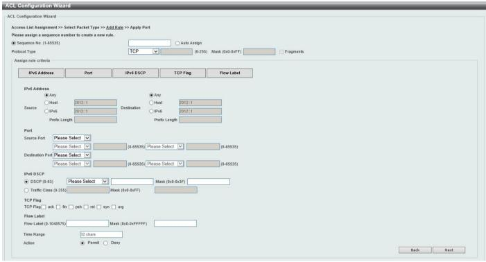
Figure 8-6 ACL Configuration Wizard (Create, Packet Type, IPv6) Window
