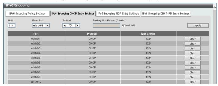
Figure 9-577 IPv6 Snooping (IPv6 Snooping DHCP Entry Settings) Window
