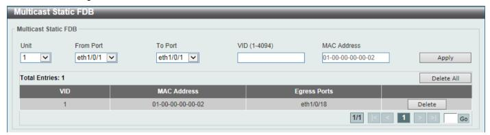
Figure 5-2 Multicast Static FDB Window
