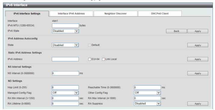
Figure 6-32 IPv6 Interface (Detail, IPv6 Interface Settings) Window
