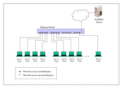
Figure 9-10 Example of Typical Port-based Configuration
