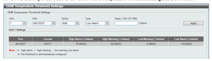
Figure 10-28 DDM Temperature Threshold Settings Window
