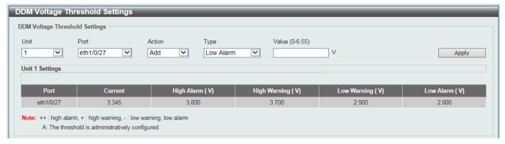
Figure 10-29 DDM Voltage Threshold Settings Window
