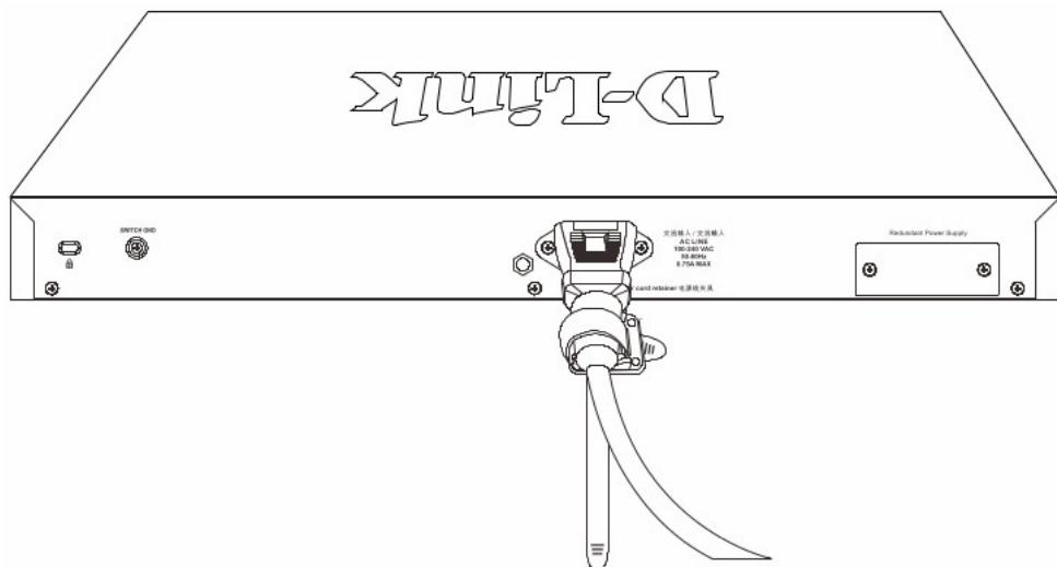
Figure 9 — Secure the power cord
