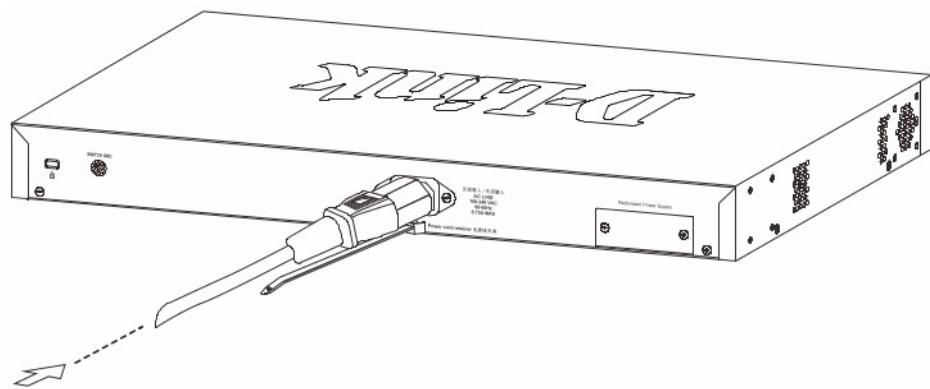
**Figure 6 — Connect the power cord to the Switch**
