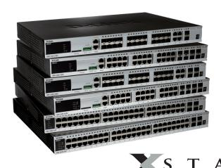
The xStack DGS-3420 Series of next generation Layer 2+ Gigabit switches deliver performance, flexibility, security, multi-layer QoS, and accessibility, along with redundant power solutions for SMBs and enterprises. With high Gigabit port densities, Gigabit SFP, 10-Gigabit SFP+ support, and advanced software solutions, these switches can act as either departmental access layer devices or aggregation switches to form a multilevel network structured with backbone and centralized highspeed servers.
