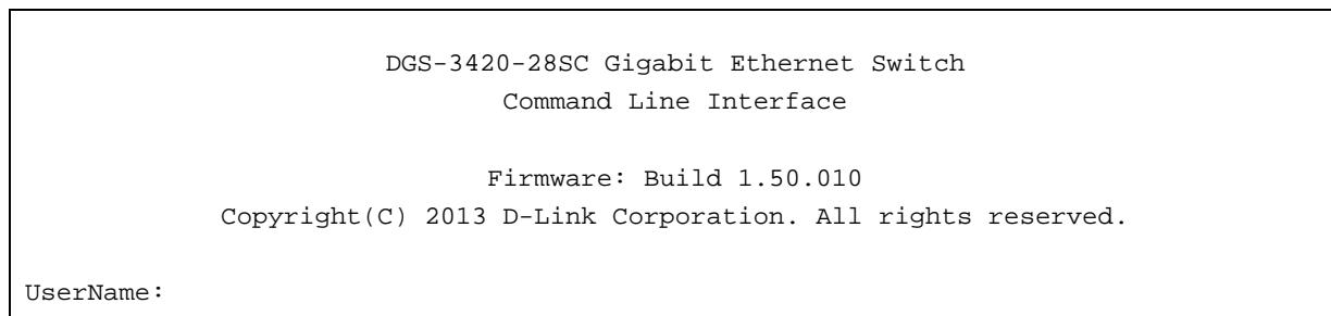
There is no initial username or password. Just press the **Enter** key twice to display the CLI input cursor – **DGS-3420-28SC:admin#**. This is the command line where all commands are input.
