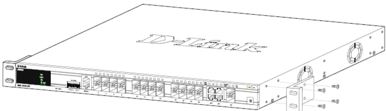
Fasten the mounting brackets in any available open space in the rack using the screws provided.
