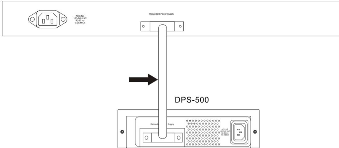
1. Insert one end of the 14-pin DC power cable into the port on the switch and the other end into the redundant power supply.
