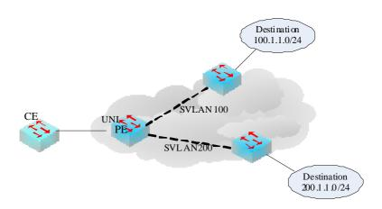
The customer packets that go to 100.1.1.0/24 will be added S-VLAN 100 and the packets that go to 200.1.1.0/24 will be added S-VLAN 200.
