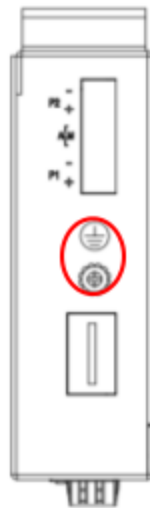
Figure 4 — The grounding screw on the switch
