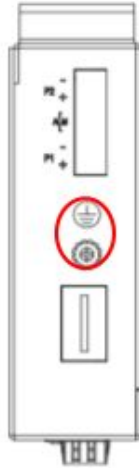
Figure 4 — The grounding screw on the switch
