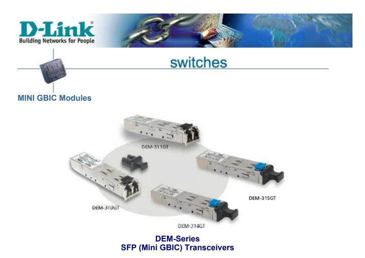
D-Link Gigabit Interface Converters (GBIC) are transceivers that connect Gigabit switches and 10/100Mbps switches with GBIC slots to Gigabit Ethernet networks, providing high-speed connections over the fiber-optic or twisted-pair cable. The fiber-optic transceivers have standard duplex LC connectors for connection compatibility.
