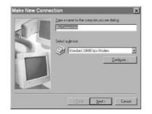
Step 14 After clicking on this new connection will display in the Dial-up Networking folder and will be used for null modem.
