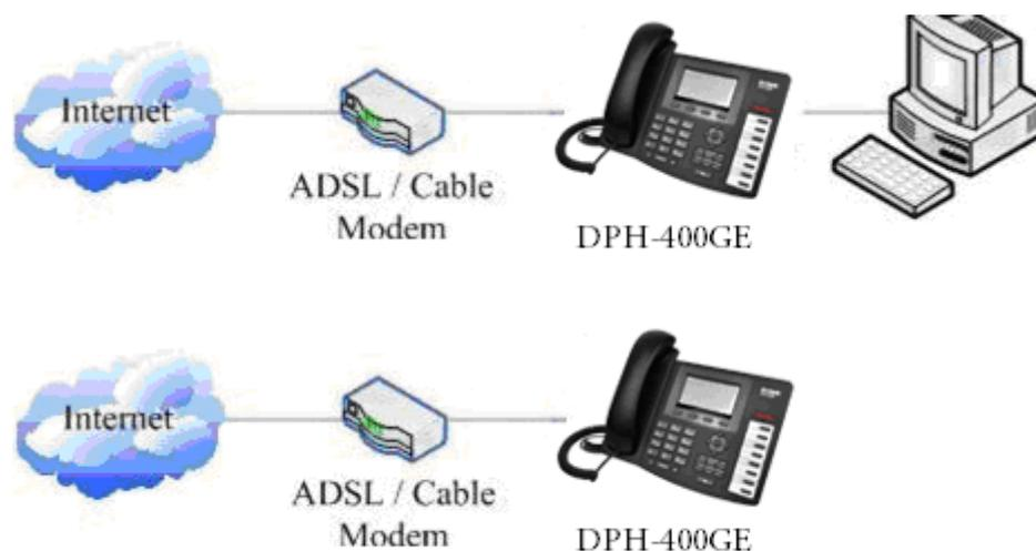
Shared network connection—Use this method if you have a single Ethernet port in your workspace with your desktop computer already connected to it. First, disconnect the Ethernet cable from the computer and attach it to the WAN port on the back of your phone. Next, use the Ethernet cable in the package to connect LAN port on the back of your phone to your desktop computer. Your IP Phone now shares a network connection with your computer. The following figure is for your reference.
