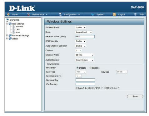
**Channel:** To change the channel, first toggle the *Auto Channel Selection* setting to **Disable**, and then use the drop-down menu to make the desired selection.
