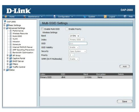
Encryption: When you select Open System, toggle between Enable and Disable. If Enable is selected, the Key Type, Key Size, Key Index (1~4), Key, and Confirm Keys must also be configured.
