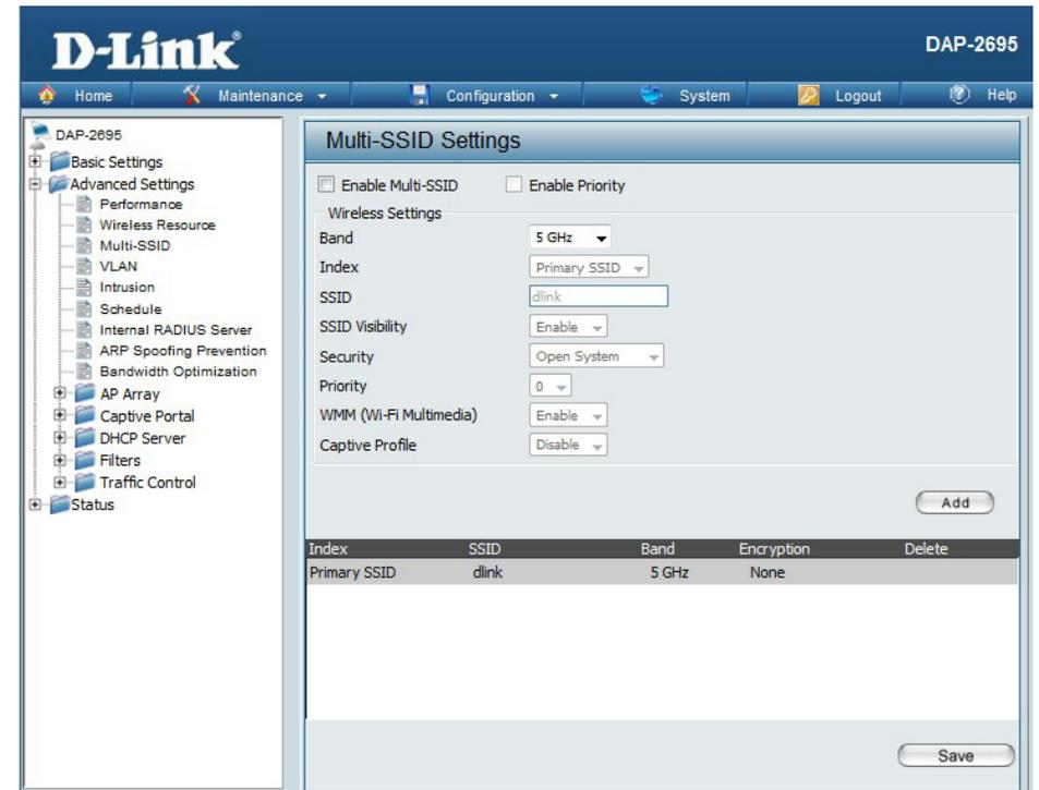
**Encryption:** When you select Open System, toggle between Enable and Disable. If Enable is selected, the Key Type, Key Size, Key Index (1~4), Key, and Confirm Keys must also be configured.
