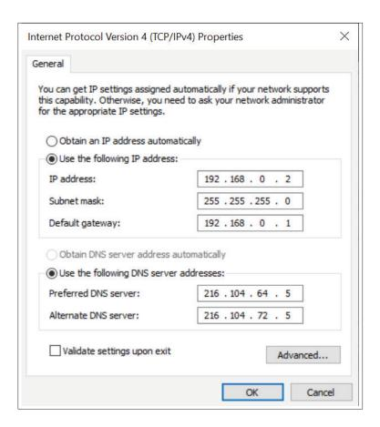
3. In the above figure, the **IP address** should be set to **192.168.0.\***. Here, \* can be any number between 1-255 (but not 50, since the DAP-3711's default IP address is **192.168.0.50**).
