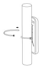
3. Wrap the metal mounting ties around the pole and thread them through the holes on the DAP-37
