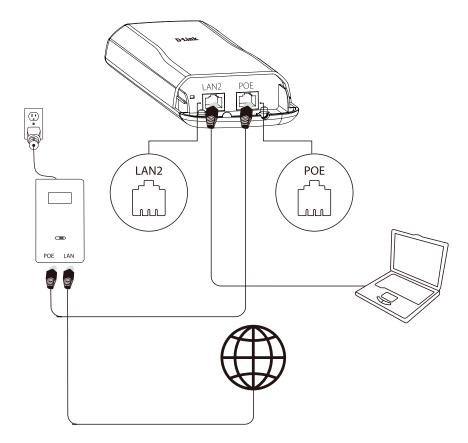
2. Ensure the computer is configured with the static IP address 192.168.0.2 and a subnet mask of 255.255.255.0.
