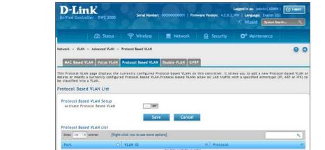
1. Go to Network > VLAN > Advanced VLAN > Protocol Based VLAN tab.
