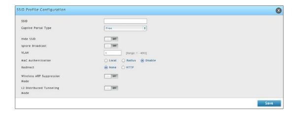
6. Click **Wireless** > **Access Point** > **AP Profile**. Click on the **AP Profile SSID** tab on the middle menu. The Access Point Profiles SSID List will appear.
