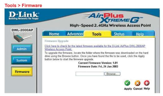
You can upgrade the firmware of the Access Point here. Make sure the firmware you want to use is on the local hard drive of the computer. Click on **Browse** to browse the local hard drive and locate the firmware to be used for the update. Please check the D-Link support site for firmware updates at http://support.dlink.com. You can download firmware upgrades to your hard drive from the D-Link support site.
