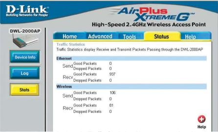
The screen above displays the Traffic Statistics. Here you can view the amount of packets that pass through the DWL-2000AP. The traffic counter will reset if the device is rebooted.
