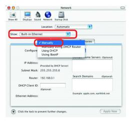
Input the Static IP Address, the Subnet Mask and the Router IP Address in the appropriate fields
