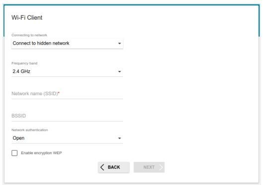
Figure 26. The page for configuring connection to a hidden network.
